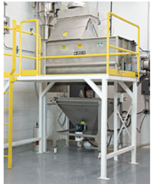
Figure 2. Blending system... A system designed to increase mixing capacity centers around a Munson ribbon blender fed via a bag dump station with dust collection and exiting into a receiving hopper with pneumatic conveying.
