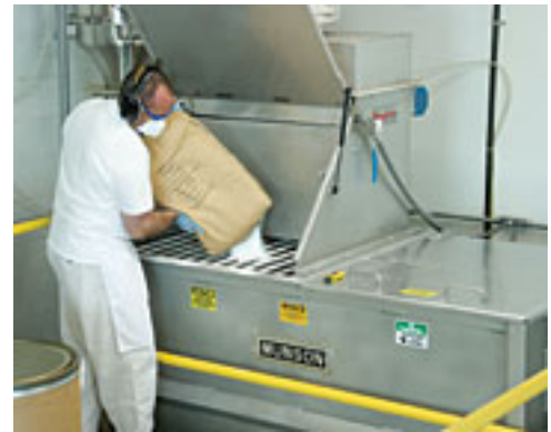
Figure 3. Bag dump station... The bag dump station includes pleated PTFE cartridge filters for dust collection and a gasketed cover for easy addition of ingredients.
