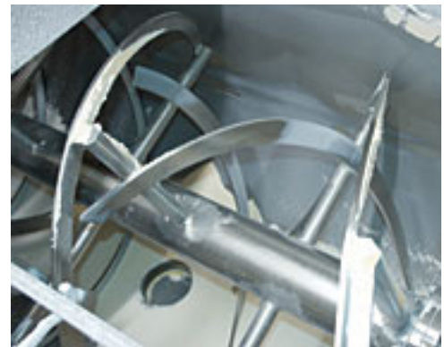
Figure 4. Ribbon blade mixing element... Ribbon blenders use helical blades with opposing pitch to achieve batch uniformity, efficiently mixing ingredients of widely varying quantities, densities, and particle sizes.
