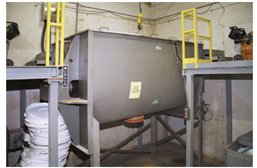
Figure 1: This 150 cu ft (4.25 cu m) paddle blender mixes most of the spices produced by J.O. Spice Company.
