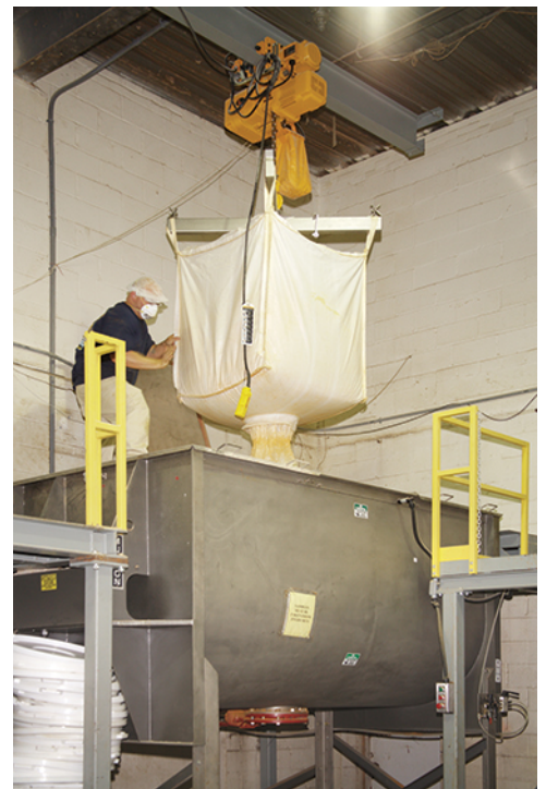
Figure 2: Most of the spice ingredients are received in 50 lb (22.7 kg) bags or boxes, but some, such as salt, come in bulk bags, which are emptied into the paddle mixer by means of a hoist.
